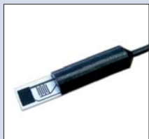
SHS - Special probe for condensation detection. Condensation sensor signals 1 when condensation causes wetting. Operation at 0...50°C Dimensions: 60mm x 10mm
