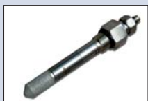
DKRF374 - Humidity/temperature probe for compressed air up to 100 bar, G3/8" thread, Operating conditions: -20...+80°C. Dimensions: 100mm x 13mm
