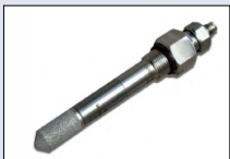
DKRF374 - Humidity/temperature probe for compressed air up to 100 bar, G3/8" thread, Operating conditions: -20...+80°C. Dimensions: 100mm x 13mm
