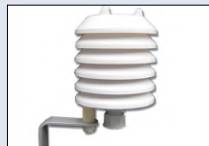
TR351 Radiation/Rain Shield suitable for probes RFT-325 and DKRF300-325. Minimizes the impact of sunlight and rain. (D=77mm/H=108mm)
