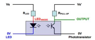
Note: The 4-wire version provides galvanic isolation between input (IR-LED) and output (Phototransistor).
